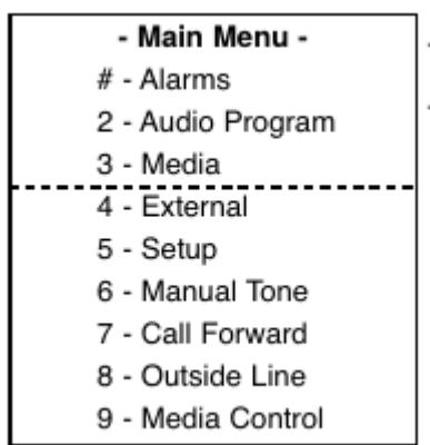
The phone will only display the top 3 (above the dotted line). In order to scroll up and down through the menu, press the (up / down) buttons.
